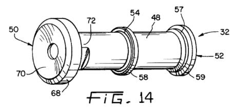
Figure 14 "is a perspective view of the button." Ex. 1013, 6:66.
