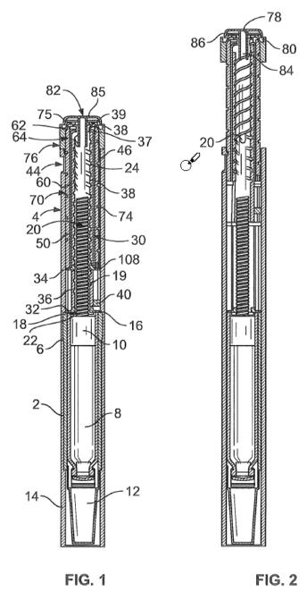
Figure 1, reproduced above, "shows a sectional view of a pen-type injector . . . in a first, cartridge full position," and Figure 2 "shows a sectional view of the pen-type injector . . . in a second, maximum first dose
