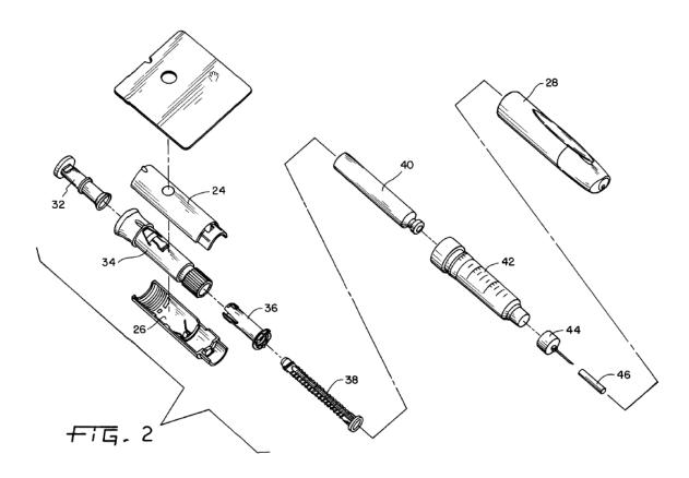
Figure 2, reproduced above, shows an exploded view of injection medication device 20. *Id.* at 6:42–43, 7:15–16. Medication device 20 includes mechanism housing 22 made from housing parts 24 and 26, button 32, dial mechanism 34, nut 36, and leadscrew 38 that forms a drive stem. *Id.* at 7:17–18, 7:32–34, 9:12–13.
