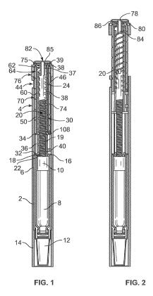
Figure 1 "shows a sectional view of a pen-type injector . . . in a first, cartridge full, position," and Figure 2 "shows a sectional view of the pen-
