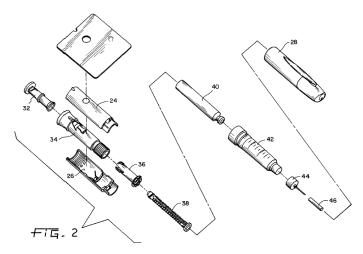
Figure 2 shows an exploded view of injection medication device 20. *Id.* at 6:42–43, 7:15–16. Medication device 20 includes mechanism housing 22 made from housing parts 24 and 26, button 32, dial mechanism 34, nut 36, and leadscrew 38 that forms a drive stem. *Id.* at 7:17–18, 7:32–34, 9:12–13.
