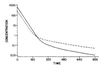
Ex. 1052, 249 (Fig. 1). The figure above shows "[t]ypical concentration-time profile in plasma (*continuous line*) and tissues (*broken line*) for a drug that is subject to high-affinity low-capacity binding in tissues." *Id*.
